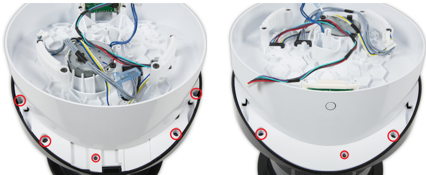
123 Remove the six 12mm T-10 and two 8mm T-6 screws from the front and rear of the Tilt plate.
