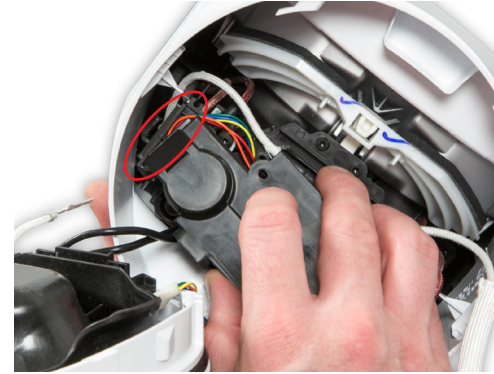
114 Carefully locate the ledge on the cover into the gap in the terminal plate. Important: it is crucial that there are no wires trapped between the cover and the plate.
